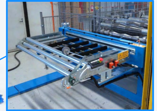
Devices for accurate sheet in-feeding. Front shear for material usage optimization.
