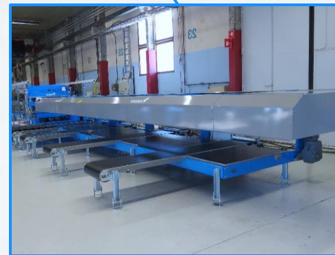
Stacking table with NC driven robotic gripper for pyramid type stacking and multi stacks.
