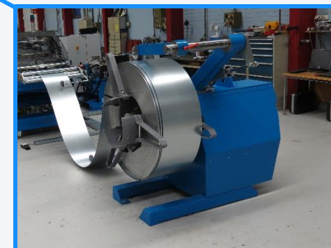
As a compact system, a 3-ton decoiler is optimal.
