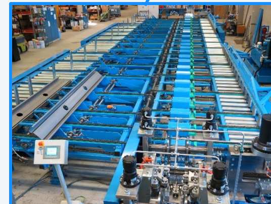
Fully automatic receiving, stacking and handling system available as an option.
